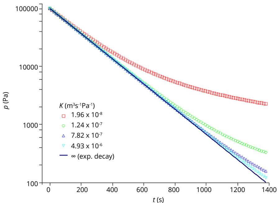
**Figure 2:** Pressure chamber for various values of  $K = \pi R^4 / (8\mu L)$ . As  $K$  increases, the pressure decay tends to exponential decay.
