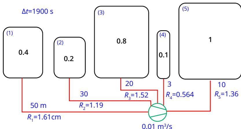
**Figure 4:** Given the positions of the chambers relative to the pump in addition to a specified evacuation time interval, one can determine the radii of the tubes that homogenize the pressure decay in all chambers as indicated.
