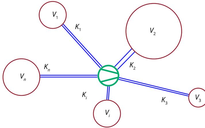
**Figure 3:** Schematics of a multi chamber vacuum system connected in parallel to a single pump.
