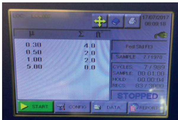
Figure 3: The control panel of Solair 1100 particle counter showing the number of particles registered after 1 minute of blowing ionized nitrogen gas at 3 bars.
