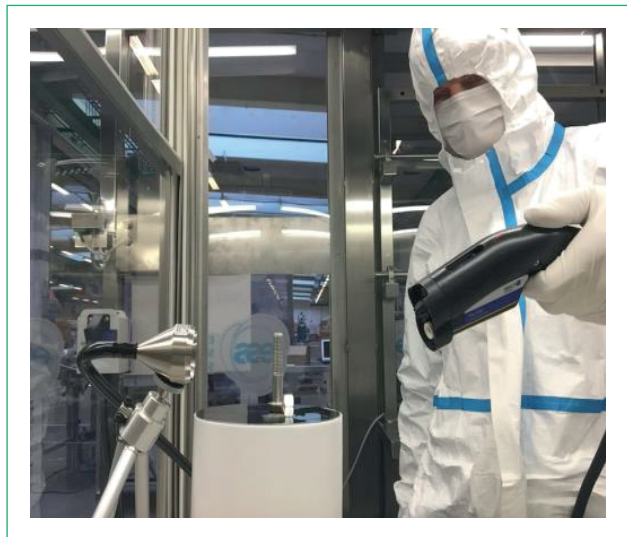
Figure 12: The operator is measuring the number of particles released by the bolt before assembly or after disassembly.
