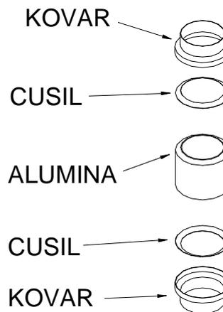
Figure 5: All view of the brazing components.
