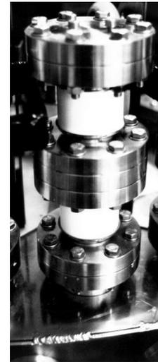
Figure 8: Photograph of the feedthrough assembled on the vacuum vessel.
