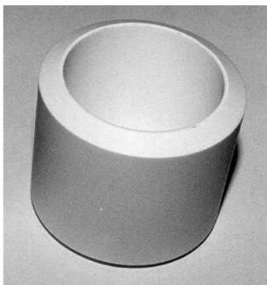
Figura 2: Photograph of a alumina tube after being submitted to the heating procedure.
