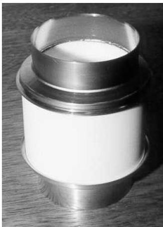
Figure 7: Photograph of one unit of feedthrough after the brazing process.
