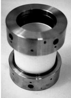
Figure 6: Capsule device used to brazing.
