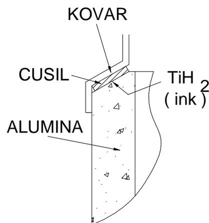
Figure 1: Sketch of the assembly for ceramic-metal joint.
