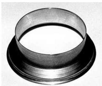
Figura 3: Photograph of the kovar metal after spouting operation.
