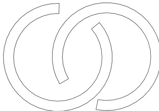
Figure 4: Sketch of the CuSil fillers used on the conic surfaces of the ceramic tubes .
