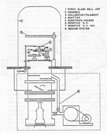
Fig.1. Scheme of the evaporator
