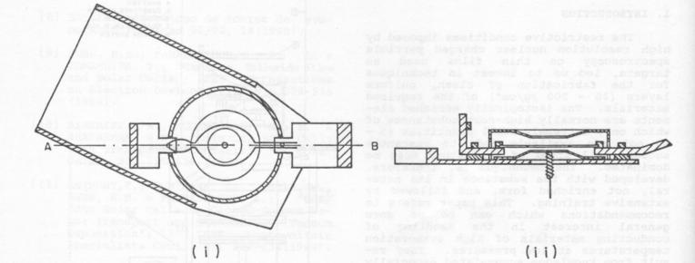
Fig.2. Detailed views of the bombarding system:
