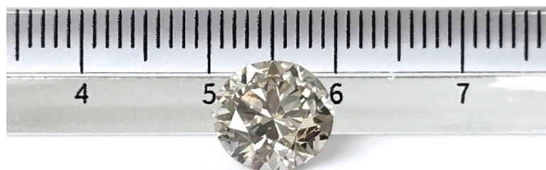
Figure 2: First gem-quality single-crystal CVD diamond produced in Brazil (2.5 ct). The crystal was grown homoepitaxially on a type Ib HPHT seed in two MPCVD stages, laser-cut, and cut and polished into a round brilliant.
