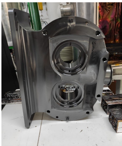
Figure 12: Large device with complex geometry coated with diamond-like carbon.
