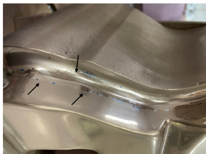
Figure 31: Loss of adhesion of arc-PVD layer on the welding area just after the process finishes.
