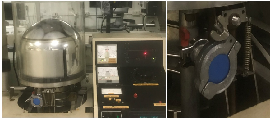
Figure 4: System used for vacuum testing. At the top, an overview of the Edwards Auto 306 system with the test flange installed. On the left, detail of the replacement of the original flange with a printed sample.
